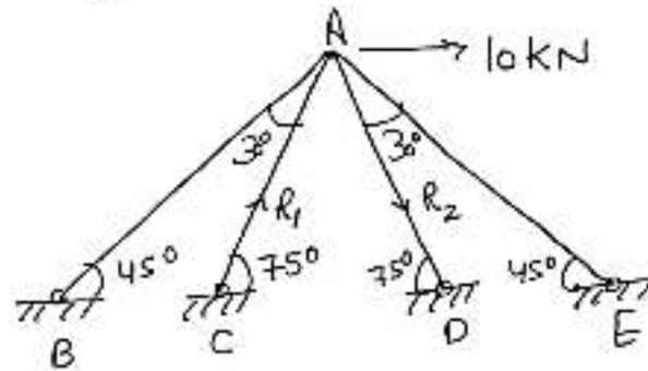
Sol • Degree of redundancy
