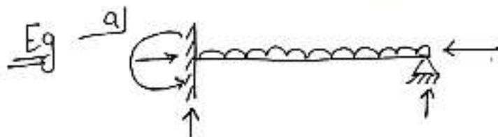
$$\begin{aligned} \text{DOI} &= 5 - 3 \\ &= 2 \end{aligned}$$
