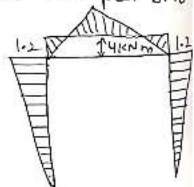
$$\frac{\partial U}{\partial H} = 0 = \frac{\partial U_{AB}}{\partial H} + \frac{\partial U_{BC}}{\partial H} + \frac{\partial U_{DC}}{\partial H} \rightarrow \textcircled{1}$$
