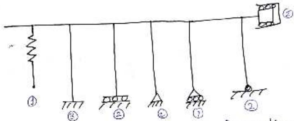
$$D_{se} = \text{Support reaction} - \text{no of equation}$$
