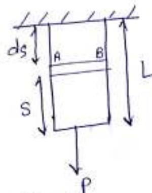
$$\text{But work done} = \frac{1}{2} \times \text{load} \times \text{extension}$$
