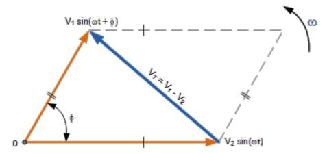
This time instead of "adding" together both the horizontal and vertical components we take them away, subtraction.
