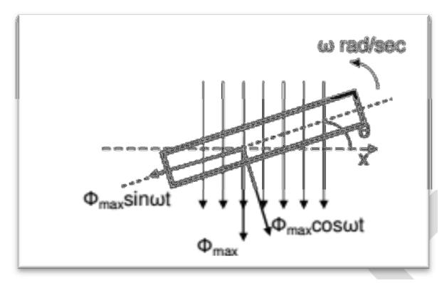
The component of flux acting along the plane of the coil does not induce any flux in the coil.
