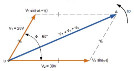
Their phasor sum  $V_1 + V_2$  can be easily found by measuring the length of the diagonal line, known as the "resultant r-vector", from the zero point to the intersection of the construction lines 0-A.
